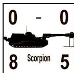
The Matilda was now retired as a front line tank but the hulls were used for various conversions. The Matilda CS was still used to support the Valentine tanks which did not have a CS version. The Scorpion was a field modified Matilda with the guns removed and a rotating flail fixed in front of the tank to detonate mines. 25 of these helped clear mines at El Alamein. These should use the same special rules as the Sherman flail.
